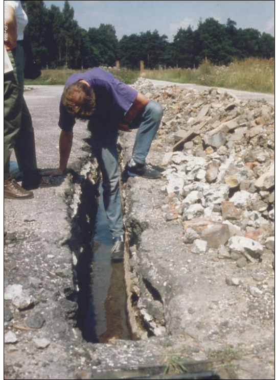
Figure 112: Groundwater level in the Birkenau Camp in August 1991 – in a construction trench with the author (center) and Anita Philipp (left) in front of the Zentralsauna : approximately 70 cm.
